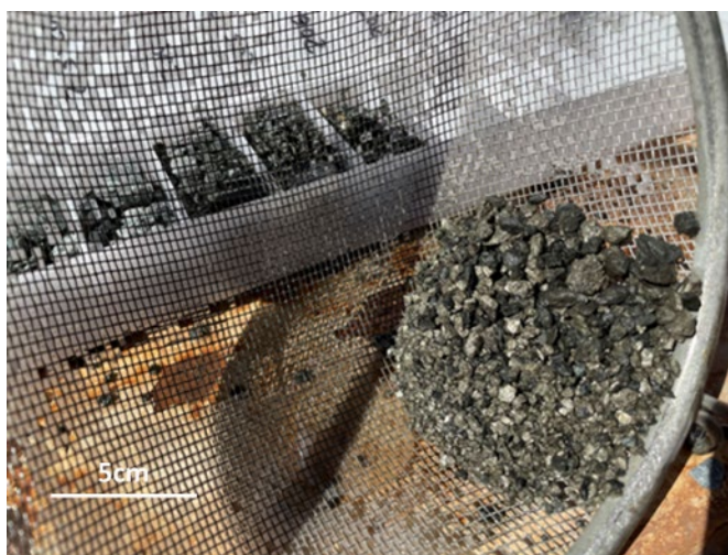
Massive sulphide chips in MIRC013 from 207-208m (pXRF 0.7% Cu and 0.2% Ni)
